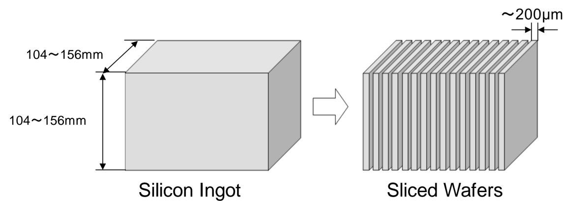
Silicon wafers for solar cells are sliced from ingot.
