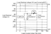
With such a load a bleeder resistance should be connected in parallel so as to allows current of more than 5mA while the unit is in the ON state. It is recommended to allow a current of more than 10mA, if possible, while the unit is in the ON state. The maximum allowable current is 200mA.
