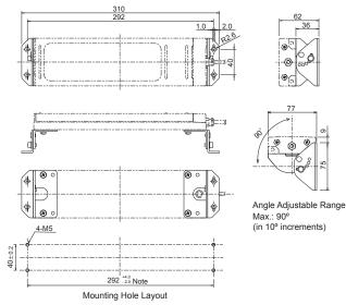
Note: This distance is the mounting centers when the outside diameter of the washer for mounting screws on the base is  $\phi$  10 mm maximum. When the washer diameter is over  $\phi$  10 mm up to  $\phi$  12 mm, the tolerance will be 292.0  $_{0.05}^{+0.05}$  mm.
