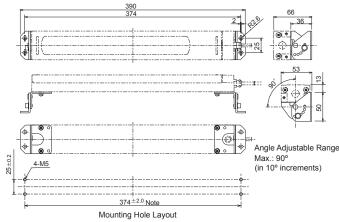
Note: This distance is the mounting centers when the outside diameter of the washer for mounting screws on the base is  $\phi$  10 mm maximum. When the washer diameter is over  $\phi$  10 mm up to  $\phi$  12 mm, the tolerance will be 374.0 % mm.
