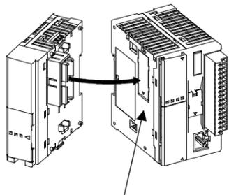
Remove the communication connector cover.
