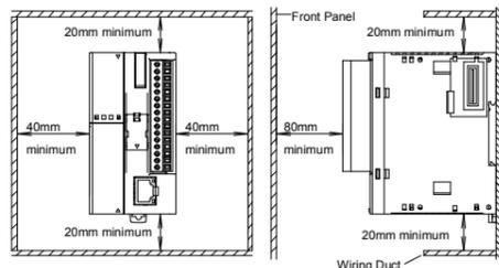
Always mount the slim type CPU modules horizontally on a vertical plane as shown above. Any other mounting directions are not allowed.
