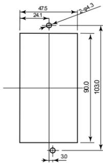
5 Installation in Control Panel & Mounting Direction
