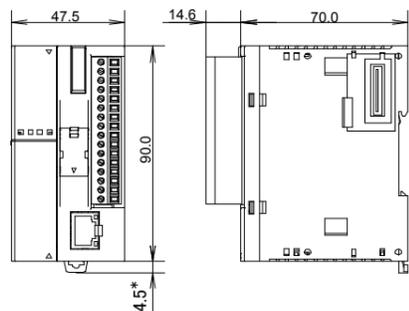
\* 8.5 mm when the clamp is pulled out. Dimensions in mm.
