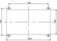
When directly mounting the SmartAXIS, tighten mounting screws with torque of 1 N·m.
