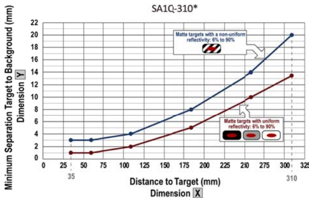
Figure 10. Minimum Object Separation Distance (90 to 6% reflectance)
