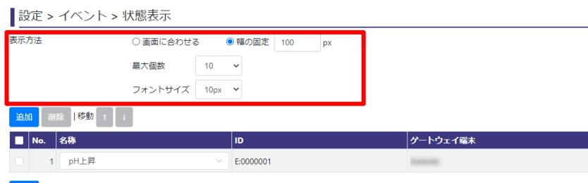
The screenshot shows the 'Status Display' configuration screen. It includes settings for 'Display Method' (选择 'Width Fixed' at 100px), 'Maximum Count' (set to 10), and 'Font Size' (set to 10px). Below this is a table with a single row for 'pH昇' with ID E:0000001 and a 'Gateway Endpoint' column. A blue button labeled '登録' (Register) is at the bottom.
