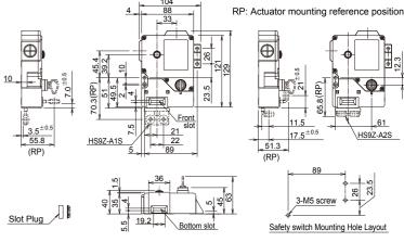
Note: Use the slot plug attached to the safety switch to close the unused actuator entry slot.
