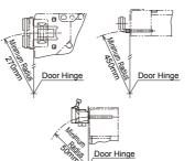
The figures shown above are based on the condition that the actuator enters and exits the actuator entry slot smoothry when the door is closed or opened. Since there may be deviation or dislocation of the hinged door, make sure of correct operation in the actual application before installation.
