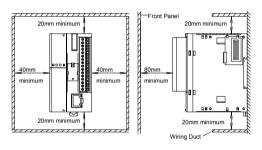
Always mount the slim type CPU modules horizontally on a vertical plane as shown above. Any other mounting directions are not allowed.
