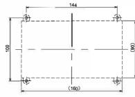
When directly mounting the SmartAXIS, tighten mounting screws with torque of 1 N·m.
