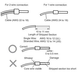
The ferrules and crimping tools below can be used. Ferrules and crimping tools made by Weidmüller or Phoenix Contact are recommended.
