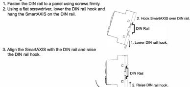
4. Secure both ends of the SmartAXIS using the DIN rail brackets
