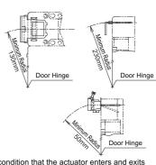
Note: The figures shown above are based on the condition that the actuator enters and exits the actuator entry slot smoothly when the door is closed or opened. Since there may be deviation or dislocation of the hinged door, make sure of correct operation in the actual application before installation
