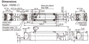
Type: HS5E-□L 18 Manual rear unlocking button Manual rear Manual unlock key Ф30 unlocking button (Supplied)
