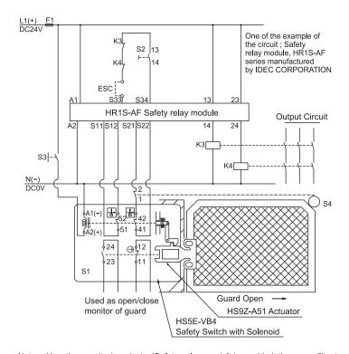
Note: Use the monitoring device(Safety relay module) provided the capavility to detect a cross short circuit. The insulation of the cable has to withstand environmental influences. If a control device other than the one shown in the draft is used, the used control device has to be equipped with a cross short circuit monitor.
