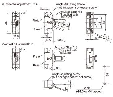
Actuator mounting hole layout
