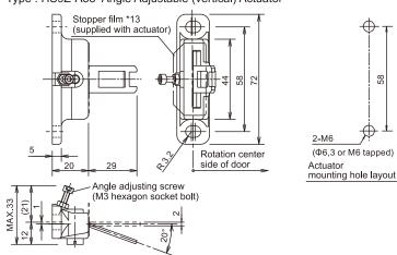
Type: HS9Z-A55 Angle Adjustable (vertical / horizontal) Actuator
