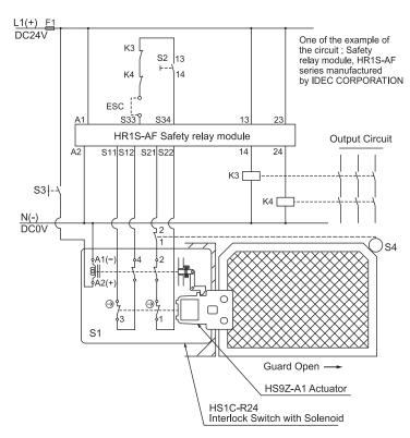
Note: Use the monitoring device(Safety relay module) provided the capability to detect a cross short circuit. The insulation of the cable has to withstand environmental influences. If a control device other than the one shown in the draft is used, the used control device has to be equipped with a cross short circuit monitor.
