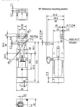
When using angle adjustable actuator (HS9Z-A15T)
