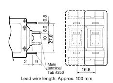
Illuminated Rocker (1-pole, with auxiliary contact) Series Trip, Switch Only
