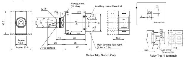
NRLY (Snap-on Mounting, Rocker) Note: The dashed lines show the 2-pole type.
