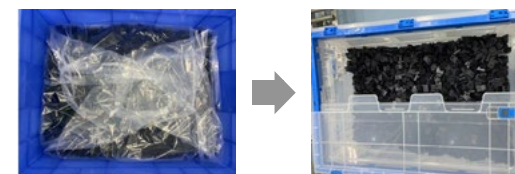
Replacement of plastic bags used in production processes with reusable plastic cases (Suzhou factory)
