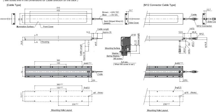
Note: Drill a hole on the panel when installing the LF1D with cable gland in the back. Make sure that the drilled hole does not damage the cable.
