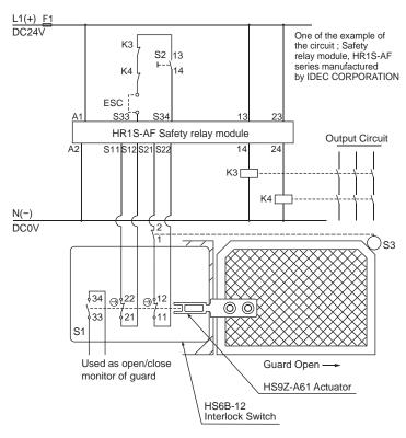
Note: Use the monitoring device(Safety relay module) provided the capability to detect a cross short circuit. The insulation of the cable has to withstand environmental influences. If a control device other than the one shown in the draft is used, the used control device has to be equipped with a cross short circuit monitor.
