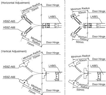
Note: The figures shown above are based on the condition that the actuator enters and exits the actuator entry slot smoothly when the door is closed or opened. Since there may be deviation or misalignment of the hinged door, make sure of correct operation in the actual application before installation.
