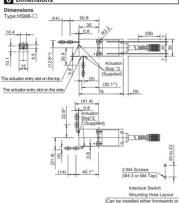
When not in use, close up the interlock switch actuator entry slots with slot plugs to prevent dust from entering.
