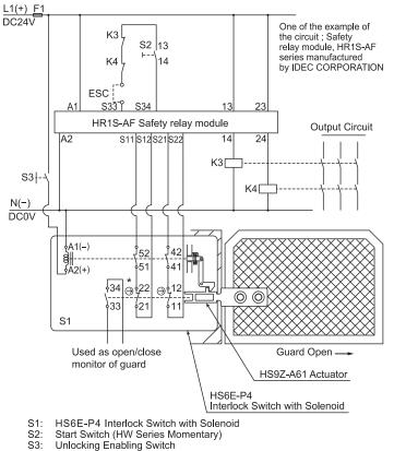
Outside fuse of safety relay module at power supply line
