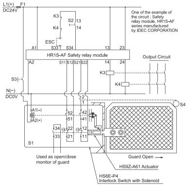
Note: Use the monitoring device(Safety relay module) provided the capability to detect a cross short circuit. The insulation of the cable has to withstand environmental influences. If a control device other than the one shown in the draft is used, the used control device has to be equipped with a cross short circuit monitor.
