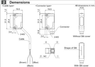
(\*4) Slit cover and connector cable are optional. (\*5) Please refer to the SA2E instruction manual for detailed dimensions.
