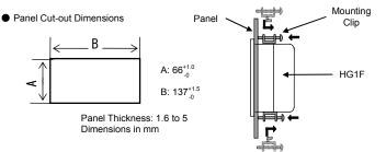
Place the HG1F in a panel cut-out and fasten with the attached mounting clips at four places to a torque of 0.12 to 0.15 N·m uniformly. Do not tighten excessively, otherwise the HG1F may be deformed or damaged.
