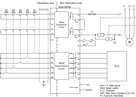
**Note.** Any possibility of a short-circuit between the conductors connected to the output terminals 13 and 24 must be excluded by constructive measures in the equipment design.
