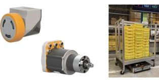
Safety Wheel Drive (left) and AMR under testing of verification at logistic centers (right)
